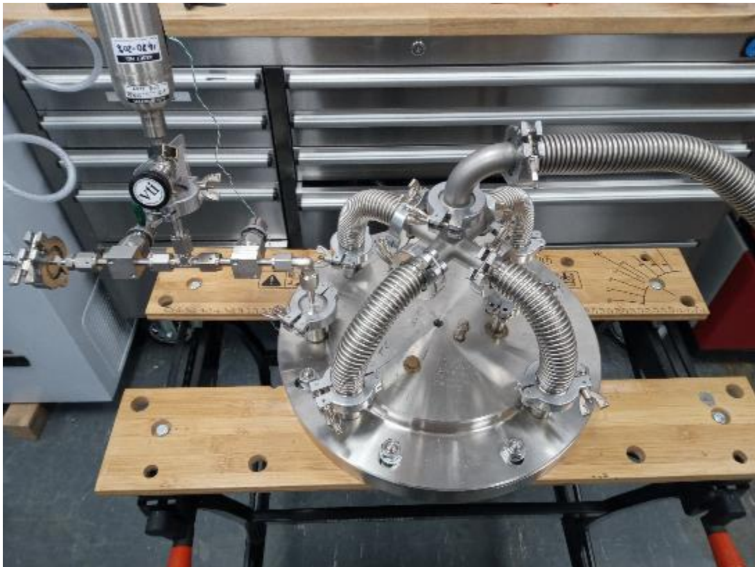
Figure 8. Four test ports at 90 degrees, all get connected to MSLD
