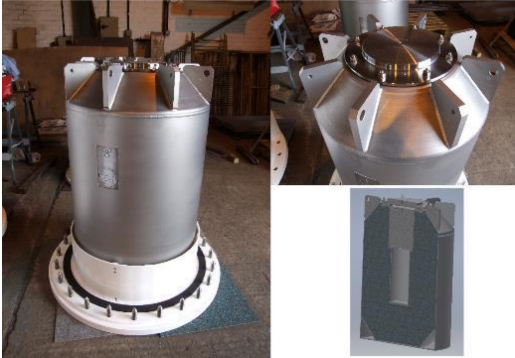
Figure 2. Flask 2774 within the 2773 casket base assembly, with a cross section depicting the internal structure and lead shielding
