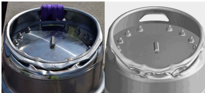
Figure 6 – Correlation between impact testing (left image) and Impact FEA (right Image) upon the 4085A Top Skirt.(9m lid edge drop)
