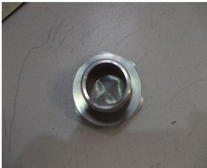
Figure 9 – Filter deformation post 20 bar burst test
