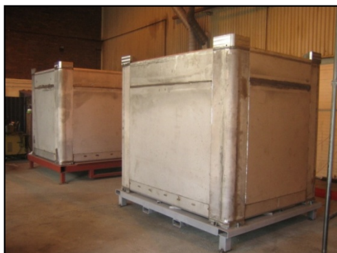
Figure 2: 2m Box Waste Package
