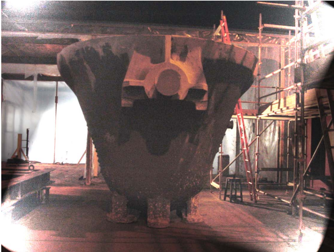
Figure 1 - Contaminated Slag Pot
