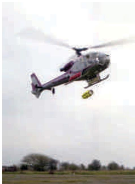
4 Package 2816C slung from helicopter before drop test
