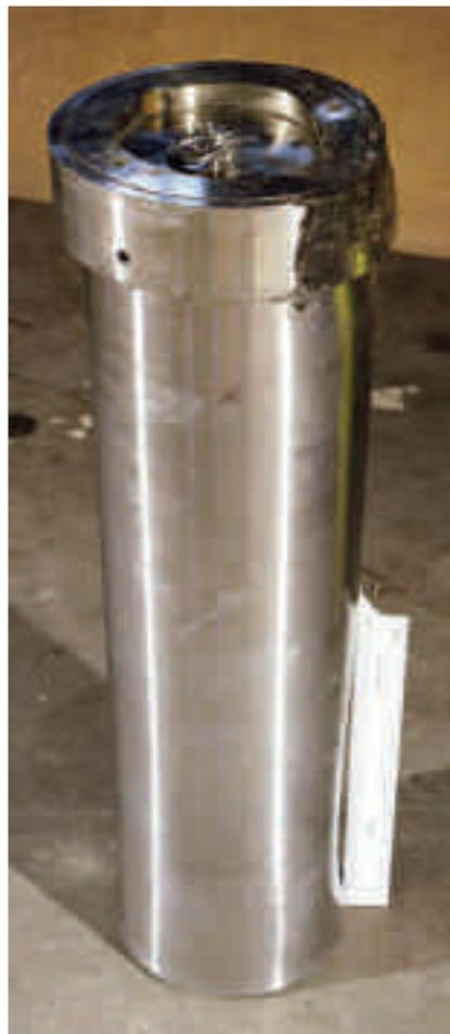
7 Containment vessel 2851 showing deformation of head and body
