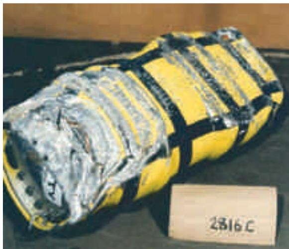
5 Package 2816C showing deformation at impact point and side
