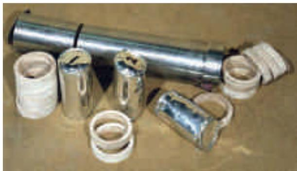
**13 Package 2816A showing condition of tinplate can following drop test**
