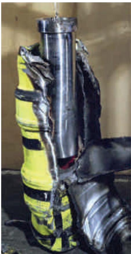
6 Package 2816C showing keg cut away to release CV
