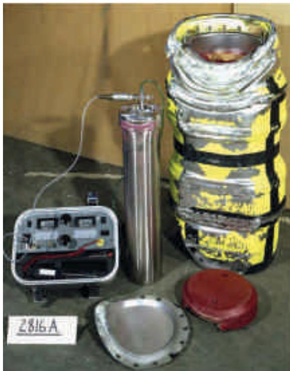
**12 SAFKEG design no. 2816C**
