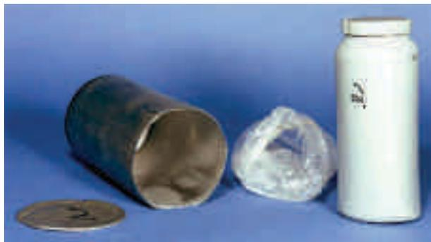
**9 Package 2816C showing condition of 3 L Bulpitt Mk II Al can following drop test**
