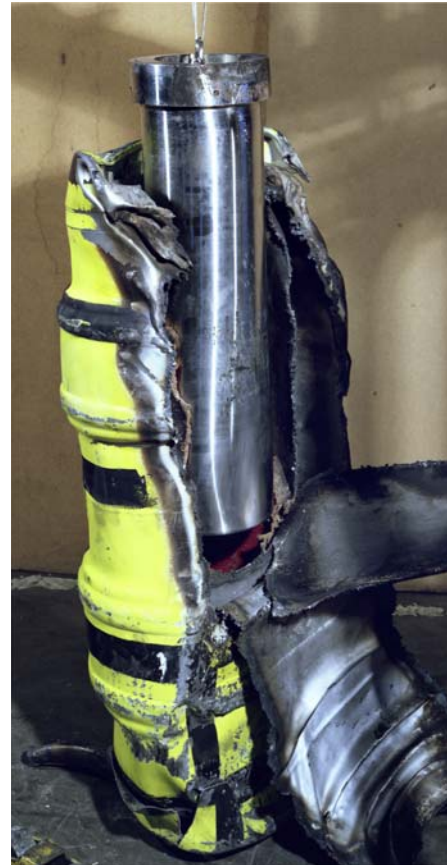
Figure 6 - Package 2816C Showing Keg cut away to release the Containment Vessel
