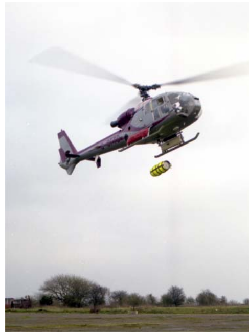
Figure 4 - Package 2816C slung from Helicopter before the Drop Test
