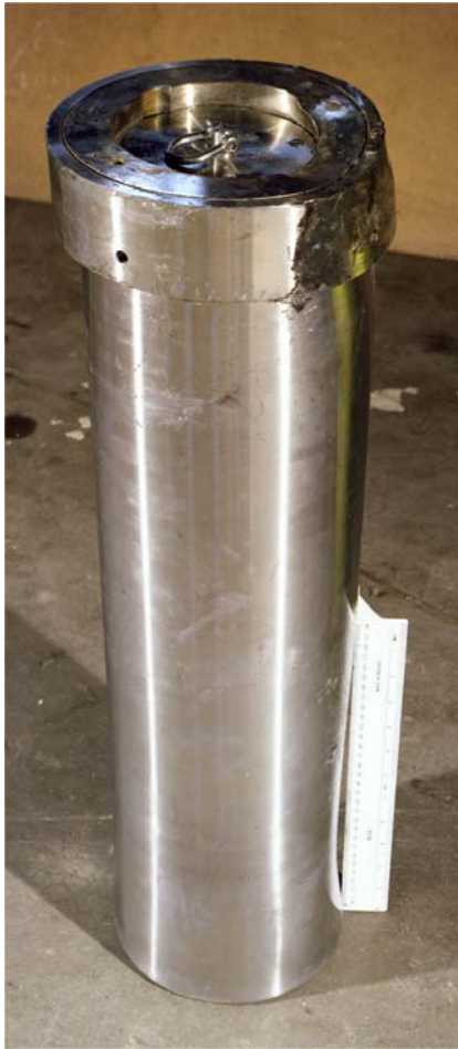
Figure 7 - Containment Vessel 2851 Showing Deformation of the Head and Body
