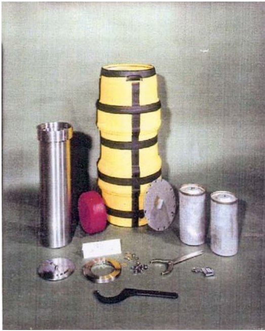
Figure 3 - Package 2816C components before assembly for testing
