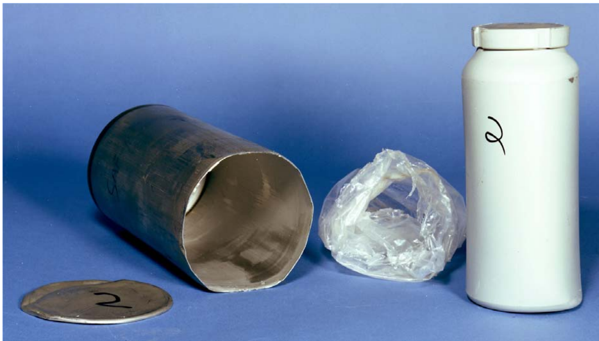
Figure 9 - Package 2816C Showing the Condition of the 3L Bulpitt Mk II Al Can following the Drop Test
