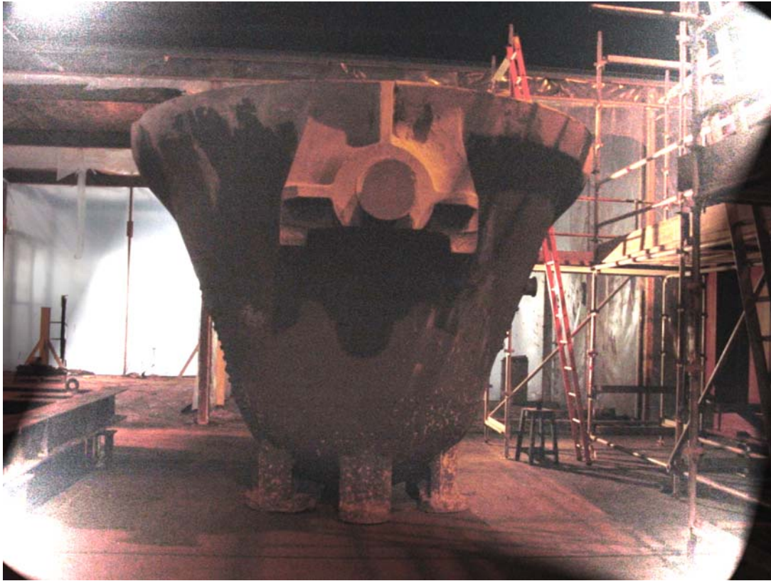
Figure 1 - Contaminated Slag Pot
